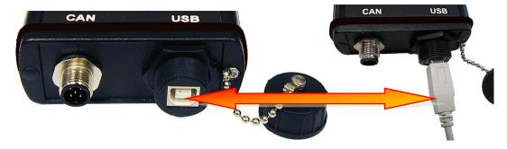
• When connecting the CCT 01 for the first time via USB to the computer, the new hardware is installed.
