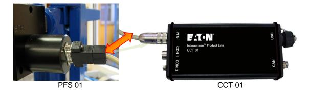
Connect the analogue outputs of the CCT 01 (CON 1 - interface) with your evaluation system. (see chapter 5.2)
